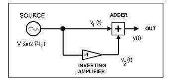
Figure 1: block diagram model of Equation 1
